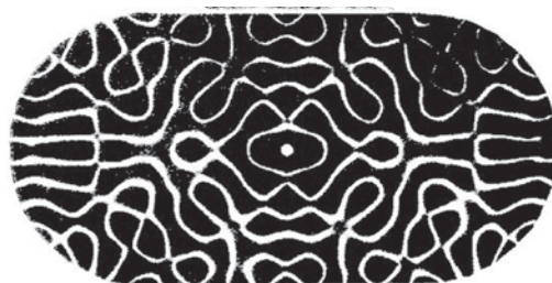
Figure 2. Chladni pattern on a metal plate
